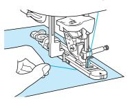
$\rightarrow$  A buttonhole starts to sew from the front of the presser foot to the back.
